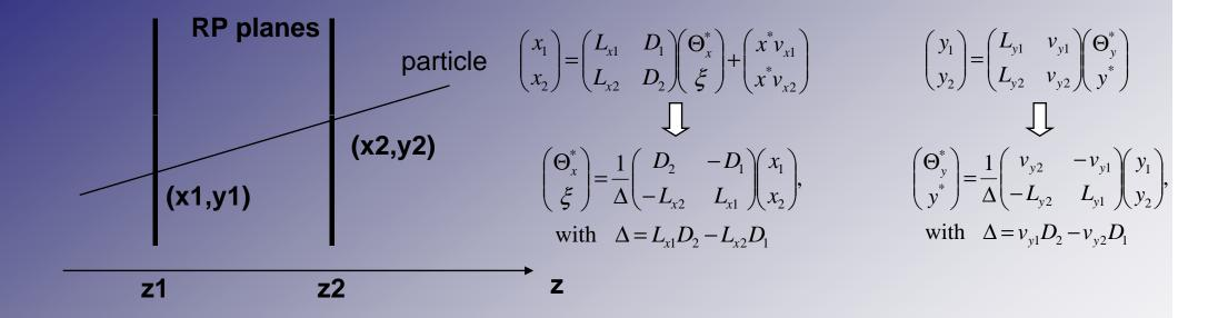
Hector reconstructs parameters of diffractive particles at IP by measurements at 2 planes. First one at the enter in RomanPot, second one at the exit. Since we can get some tracks (Reco/Sim Hits) from Sasha's Sim/RecoRP420 we can reconstruct kinematics at IP and store this information (*DiffParticleCollection*) in to *edm::Event* (ROOT file) for future using in physical analysis.
